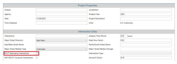
The Intersection Type dropdown will now become editable. The default selection is RCUT with Stop Signs. Note: Activating the RCUT Alternative Intersection checkbox adds three new input sections to TWSC titled Conventional Intersection, RCUT Main Intersection, and U-Turn Crossovers, as displayed below.
