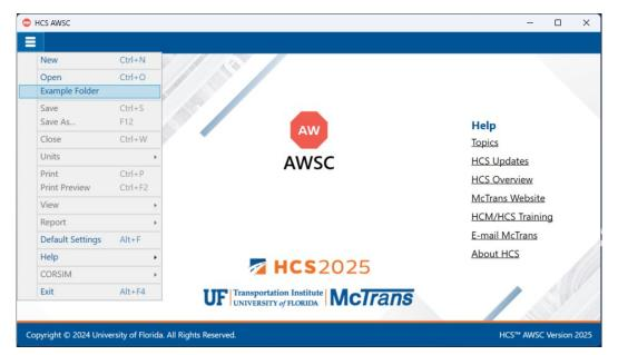
f. Selecting "Example Folder..." from the Start screen; this can be found below in the red box. Opening the example folder will open the path of the HCS example files in File Explorer. The desired example file can be double-clicked or right-clicked and selecting 'Open', which will open the example file in the AWSC program.
