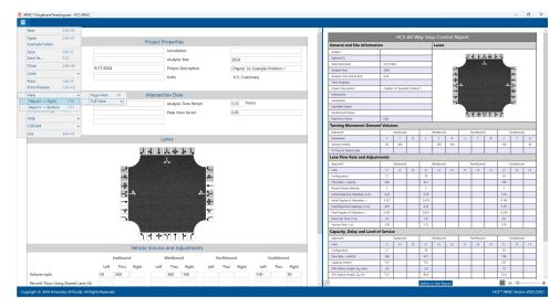
iii. To switch to Full View with the report on the bottom of the screen, select File > View > Full View > Report -> Bottom from the main menu; this can be found by selecting the three lines in the top left-hand corner of the screen, hovering over "View", hovering over "Full View", and then selecting "Report -> Bottom".
